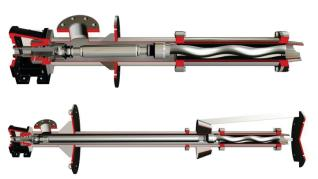
This is a vertical model designed for pumping from a tank or well and is usually immersed directly into the product being pumped. There are two versions available; a short option and a long version with removable inlet and downhole plate.
