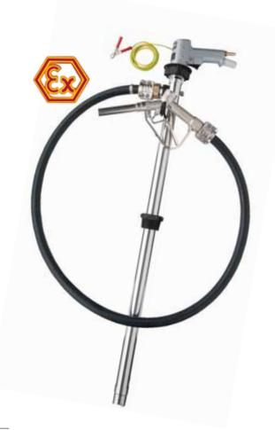
Delivery rate max. 240 l/min, delivery head max. 13 m.\* When using the pump with a discharge hose and a hand tap, the delivery rate will be approx. 55 l/min.
