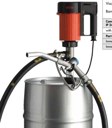
Delivery rate max. 220 l/min, delivery head max. 12 m.\* When using the pump with a discharge hose and a hand tap, the delivery rate will be approx. 80 l/min.
