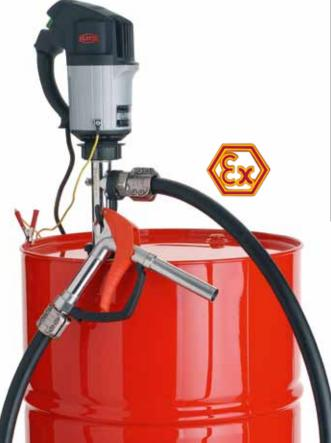
Delivery rate max. 200 l/min, delivery head max. 9,5 m.\* When using the pump with a discharge hose and a hand tap, the delivery rate will be approx. 50 l/min.
