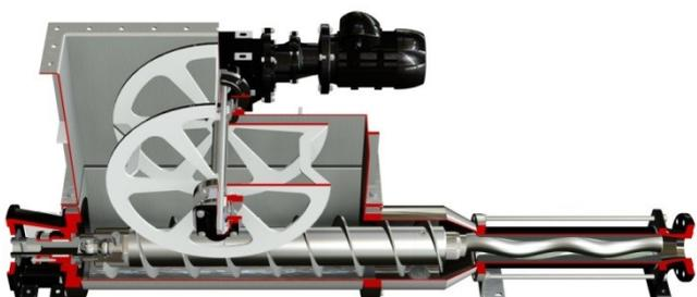
This model features a rectangular hopper, joint protection sleeve and an enlarged auger feed screw to move the product to the hydraulic part. A "B" Module is installed on the hopper which feeds the screw by means of a wheel device to prevent bridging. Suitable for pumping non-flowing materials with up to 40% solids content prone to bridging and plasticizing.
