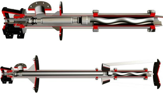
Vertical Series developed for pumping from tanks and wells immersed directly in the product to be pumped. The length can be adapted to suit the installation requirements. The stainless steel version (AISI 304 or AISI 316) is supplied with a stator jacket as standard to prevent corrosion of the stator. Two standard configurations are available: the short version and the long version with removable inlet and downhole plate.
