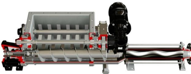
Model featuring a hopper with double bridge breaker shaft, joint protective sleeve and enlarged auger feed screw to move the product to the hydraulic part. Suitable for pumping highly viscous, non-flowing materials with up to 35% solids content prone to bridging or in blocks.
