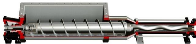
Model featuring a rectangular hopper, with joint protection sleeve and enlarged auger feed screw to move the product to the hydraulic part. Suitable for pumping high viscosity materials with low flowability and up to 28% solids content not prone to bridging.
