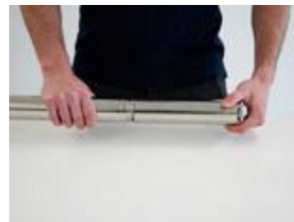
Unscrew stator housing
