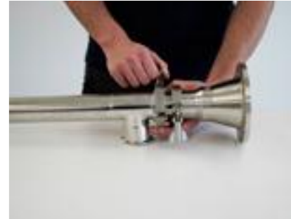
Open clamp on pump tube
